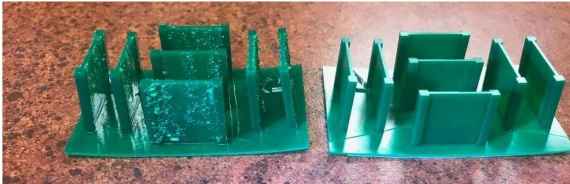
*(Picture 4) Left - print results with smears and/or smudges on optic glass*
