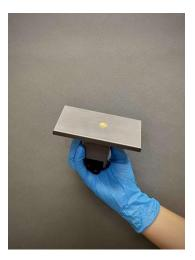
Figure 1: Proper amount of wax on build table
