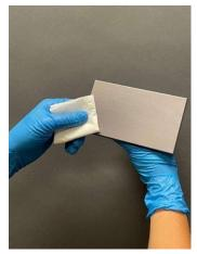
Figure 3: Build table with wax applied before buffing
