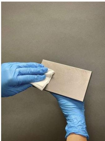
Figure 2: Wax application to build table
