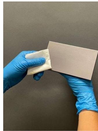
Figure 3: Build table with wax applied before buffing
