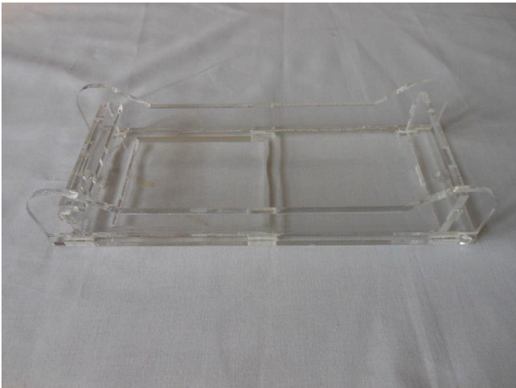
Resin VAT, VAT-01 (Clear Acrylic with PDMS floor coating)
