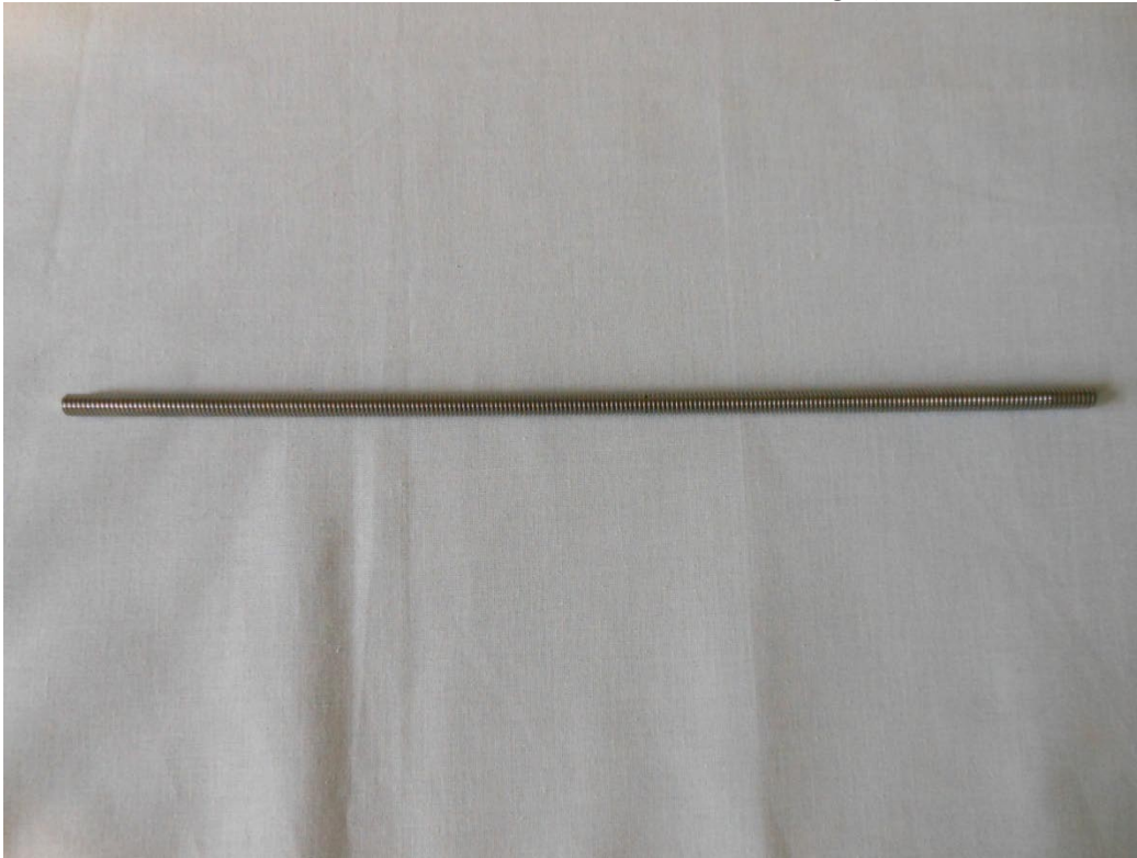
Z Axis Lead Screw, 6350K133-A (11.125" length)
