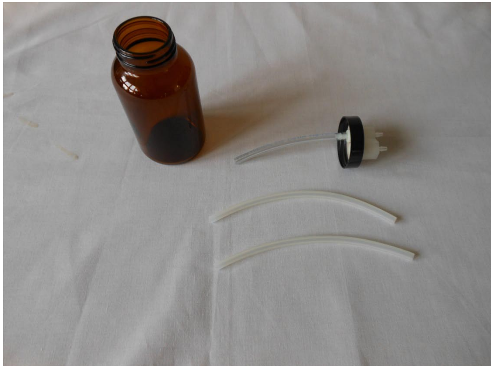
Resin Reserve Bottle, internal vent tube, cap, external vent & feed tubes
