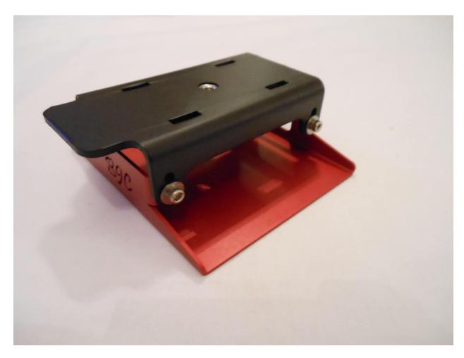
You only need to hand tighten the four screws. The slots allow for vertical adjustment when calibrating the table against the bottom of the vat. They will be fully tightened during that calibration procedure.
