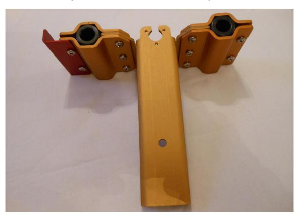
Securely tighten the six inner most screws. Do not over tighten the four outer screws, they need only provide sufficient clamping force to hold the bearings.
