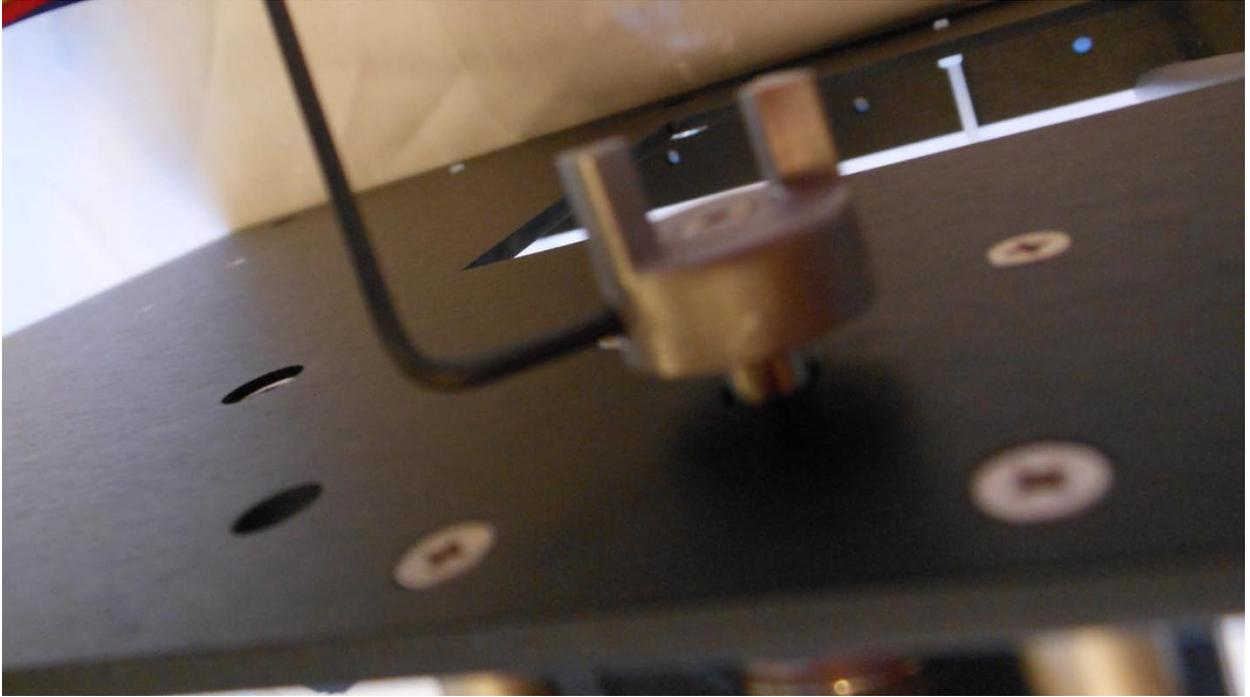
Use the hex wrench to secure the motor coupler. Motor shaft should be flush with couper as shown.
