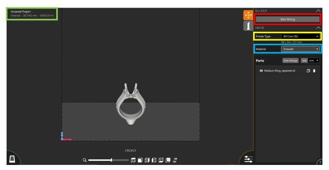
1.0 Model Layout and Orientation: In B9Create 1.0, the model manipulation tools are across the top middle of the view window (Red), the Duplicate and Remove buttons are above the Model List (Yellow), and the Model Information (Green) is under the Model List. The Snap to Floor button (Blue) is located above the Perspective Snap Tools.
