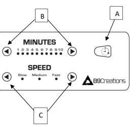
The Start/Stop button (A) starts or stops a cleaning cycle and is located on the right side of the control interface. A cleaning cycle is characterized by the 3D printed parts in the inner container being submerged in isopropyl alcohol that is stirred at a specified speed for a specified duration.
